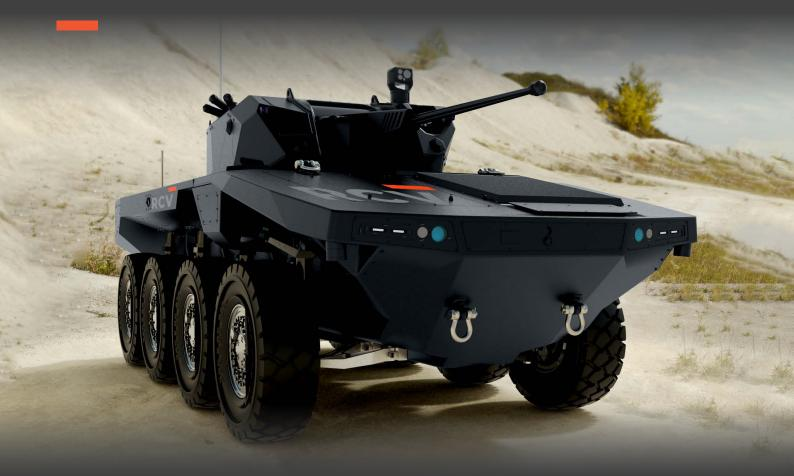
This Robotic Combat Vehicle with amphibious capabilities, rapid acceleration, top speed of 110km/h, small turning radius and low profile for stealth operations provides planners with a high-performance vehicle. Customisable for either manned or unmanned operation and all-electric or hybrid motor, the RCV is ready for any tactical challenge.
