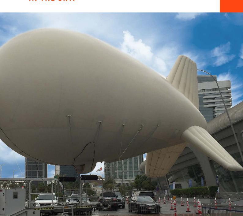
This lighter-than-air platform features a tethered, stationary unmanned mooring system in three sizes: 200m<sup>3</sup>, 300m<sup>3</sup> and 400m<sup>3</sup>. Developed in the UAE, this system is built to meet the distinctive requirements of the region, including its extreme climate. ADASI's Aerostat is designed to deliver exceptional performance at heights up to 1,500 feet above sea level. The tether delivers sustained power supply to airborne payloads.
