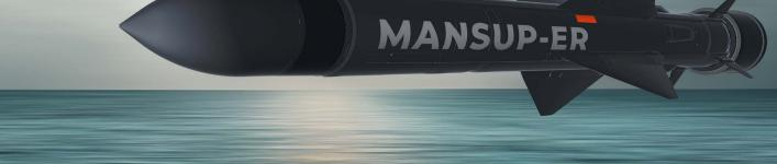
The MANSUP-ER is a versatile, long-range, surface-to-surface antiship missile system with land attack capability. Not only does the system offer adaptive sea skimming, but also unlimited overland flight, terminal manoeuvres, and simultaneous (time on target) missiles attack.
