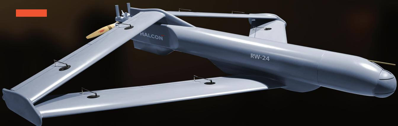
The HALCON RW-24 is a smart loitering munition that delivers autonomous ground strike capabilities against various types of targets. As part of its precision delivery, the RW-24 navigation and flight control system uses Global Navigation Satellite System (GNSS), which combines GPS, GLONASS and other satellite-based navigation systems.
