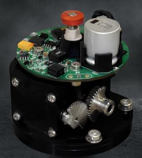
An electro-mechanical fuze with Point Detonation mode designed for use on gravity release weapon and can be fitted on any standard mortar interface.
