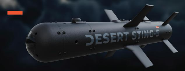
The Desert Sting is a family of light weight, air platform released, precision guided, glide weapons (GGW). The DS-5 is differentiated by weight and warhead size.
