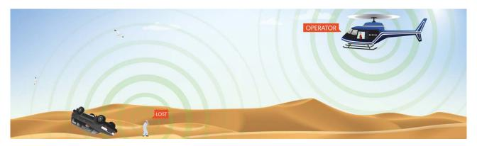
ACTIVECELL-SAR, mounted on either a manned or unmanned aircraft, enables search and rescue teams to scan large areas to find lost, missing, or injured individuals by identifying signals emitted from their mobile devices.
